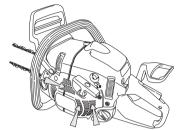
IMPORTANT! In order to maintain operation of the centrifugal cleaning system it must be regularly maintained. Clean the air intake to the starter, the fins on the flywheel, the space around the flywheel, inlet pipe and carburetor compartment.
